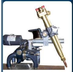
Allows both horizontal and vertical adjustment of the torch in relationship to the pipe surface.
