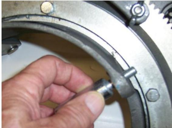
Picture 2 – Installation of Spacer Bolt
