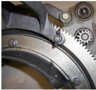
**Picture 6 – Installation of the Wing Nut**
