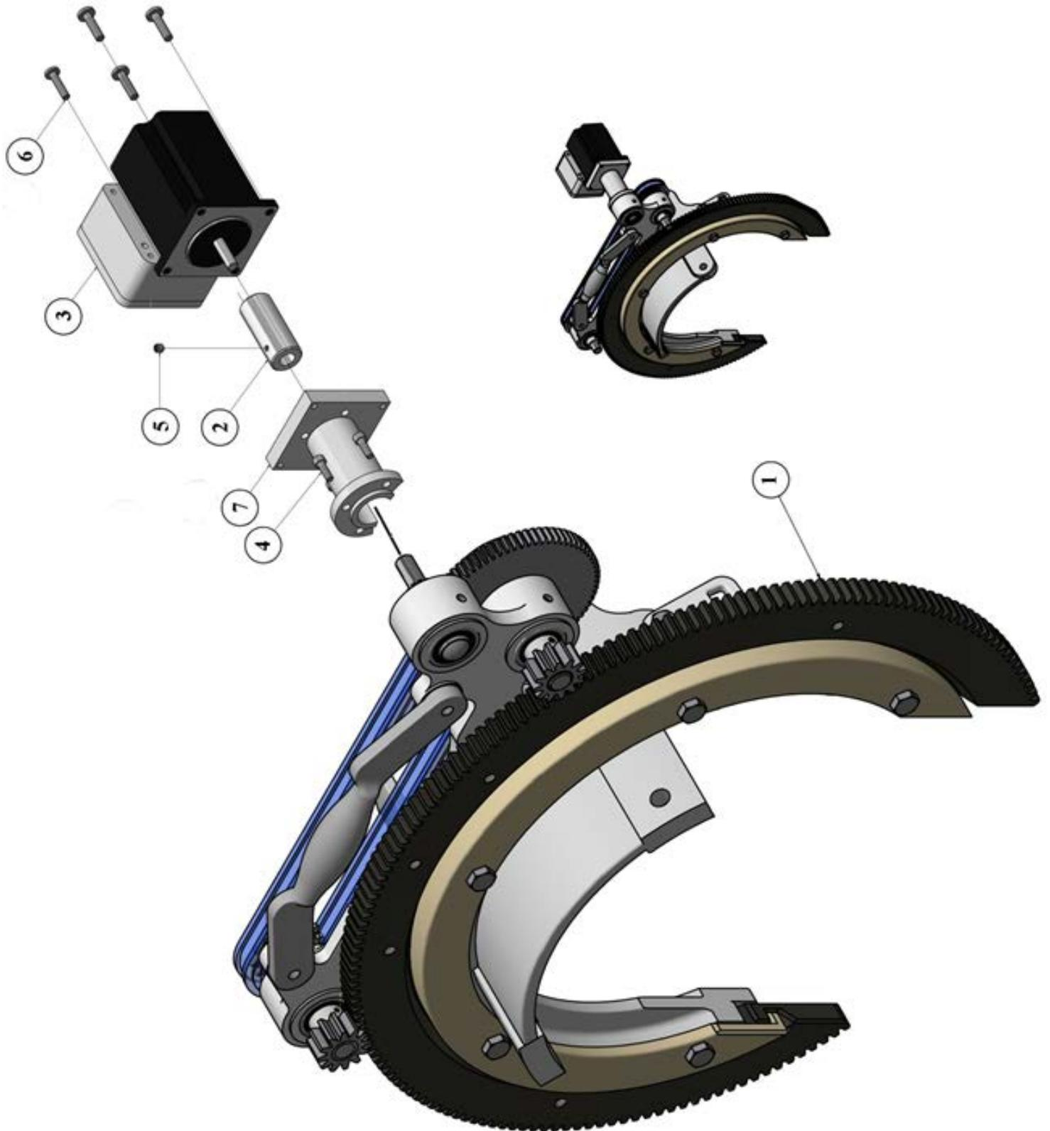
**Table 8 – Motorized 1SA Saddle Machine Parts Identification**
